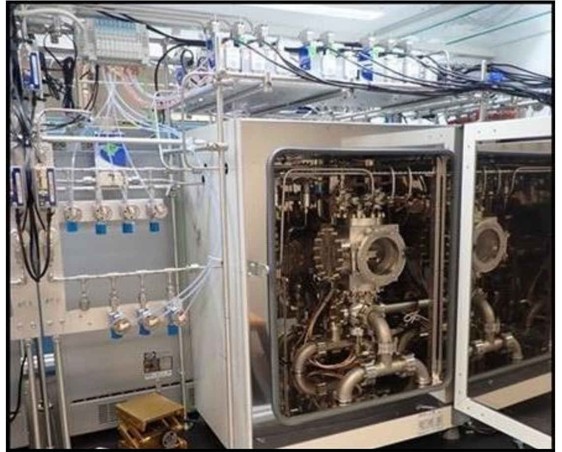
One of the two new ALD reactors . Featured here is the reaction chamber, attachment points for room temperature bubblers, and mass flow controllers for gas delivery.
