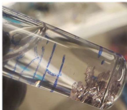
Metal precipitate from a solution-state reactivity test.
