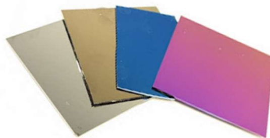
ALD-deposited Al 2 O 3 thin films of varied thicknesses.
